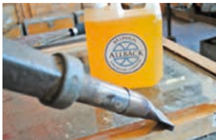
If you heat the oil with hot air, you can paint immediately.
