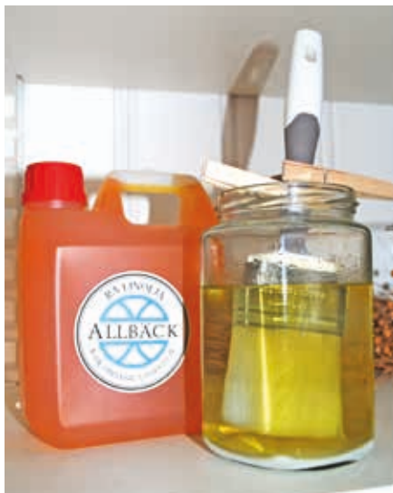
Keep brushes hanging in a jar of raw linseed oil. This oil can be reused for impregnation.
